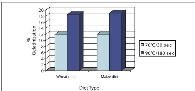
Figure 5 clearly shows that increased conditioning time and temperature increases gelatinization in feed, regardless of the cereal base used. The process of gelatinization creates natural ‘glues’ which allows the feed particles to compress tightly and adhere to each other when passing through the pellet die. Optimal ‘cooking’ of feed will result in more durable pellets and reduce levels of fines (Figure 6).
