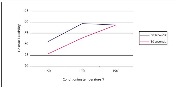
As the conditioning time and temperature was increased, the pellet durability increased (as expressed by a Holman Durability Index).
