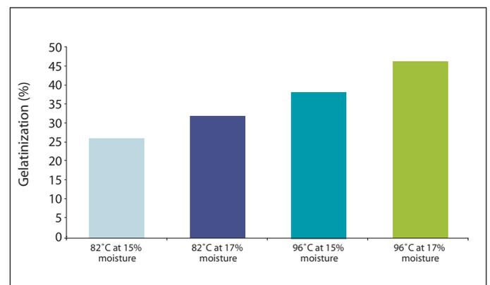
Some feed additives can also improve the conditioning process; new moisture and surfactant technologies allow the addition of moisture at the mixer or conditioning chamber which can greatly improve feed pellet quality. The addition of the moisture and the improved pellet quality has
